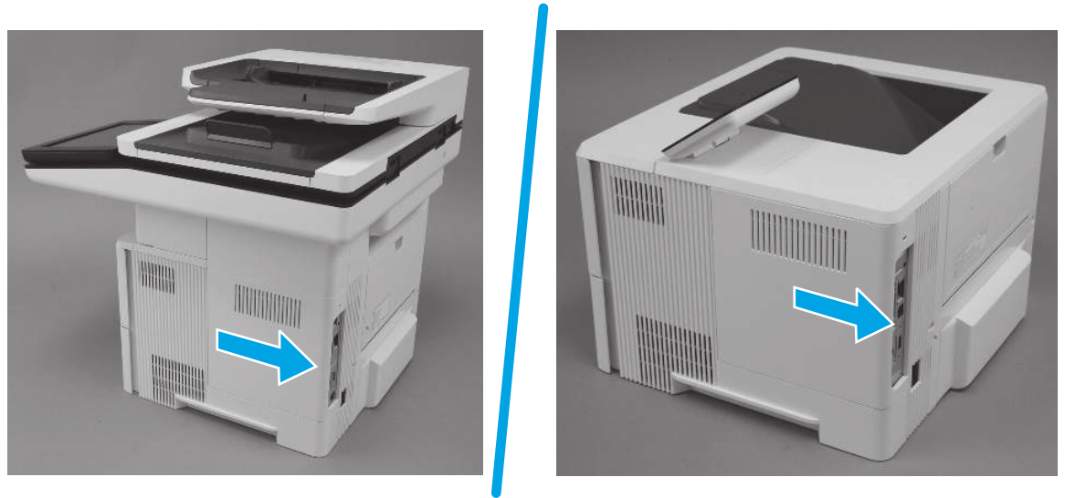
Figure 4-451 Remove the formatter cover (M506/E50045/M507/E50145/M527/E52545/M528/E52645)
