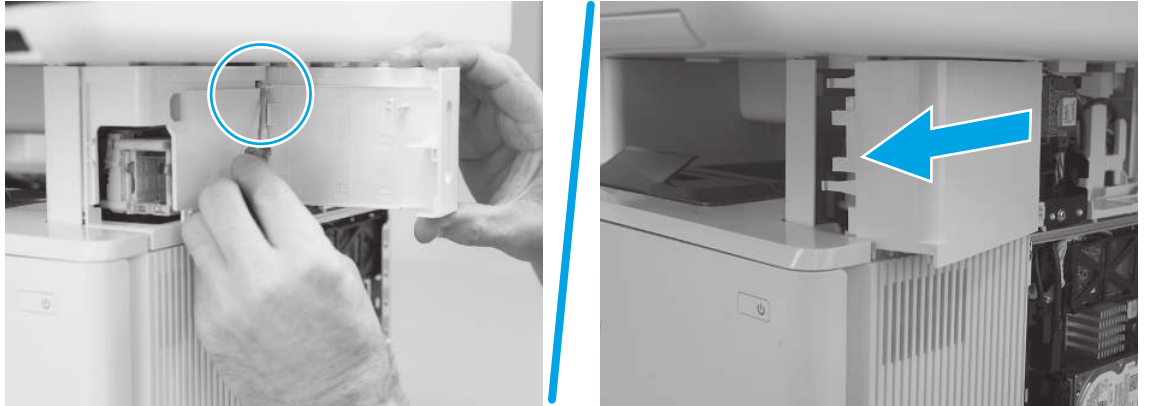
Figure 4-410 Release the upper hinge or remove the cover
