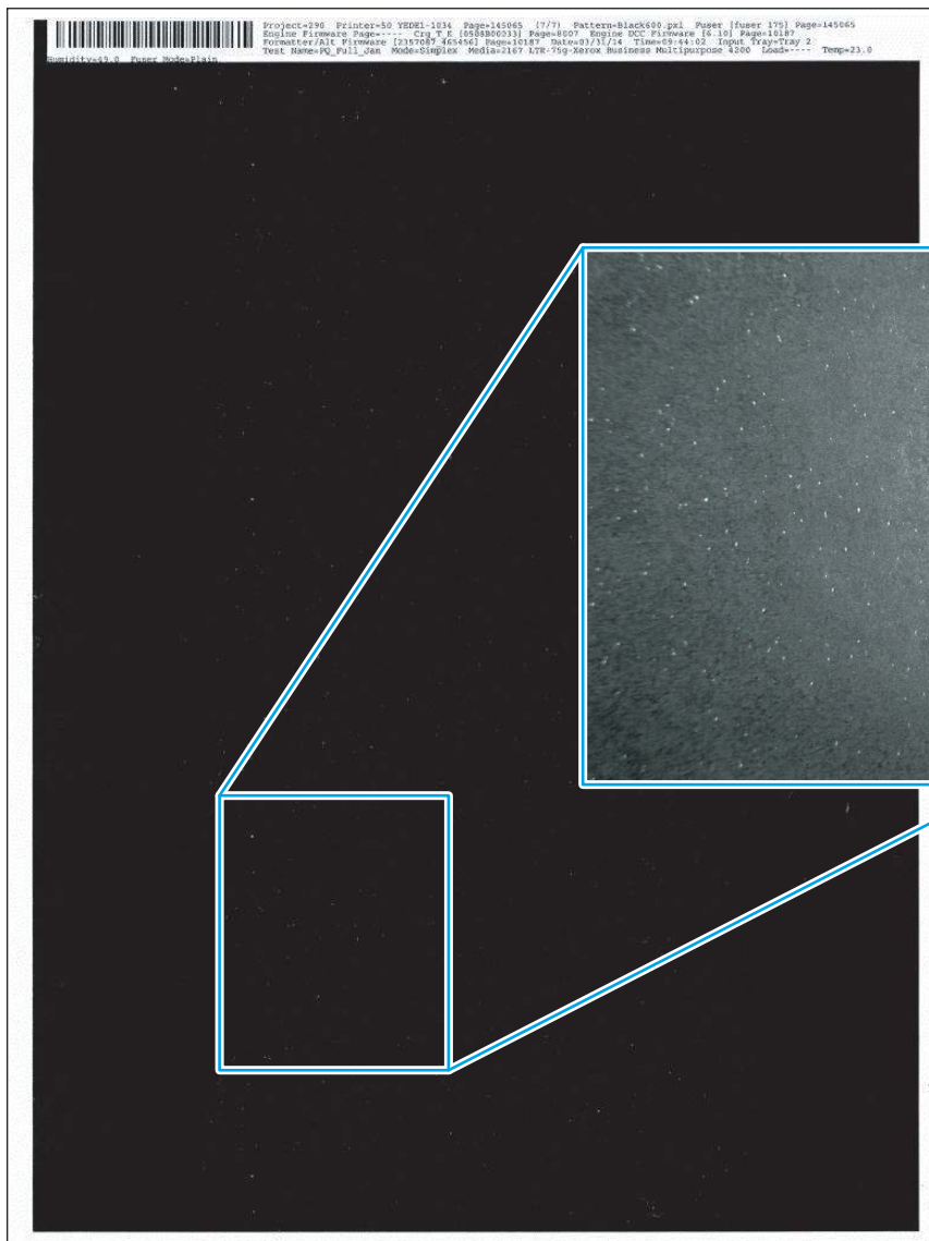
Figure 3-93 Rain-toner attached to the OPC
