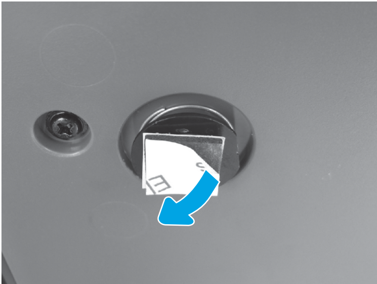
Figure 4-92 White backing adhesive squares
