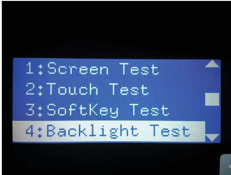
Figure 3-41 Open the backlight test
