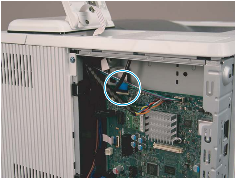
Figure 4-1289 Disconnect one FFC (M507/E50145)
