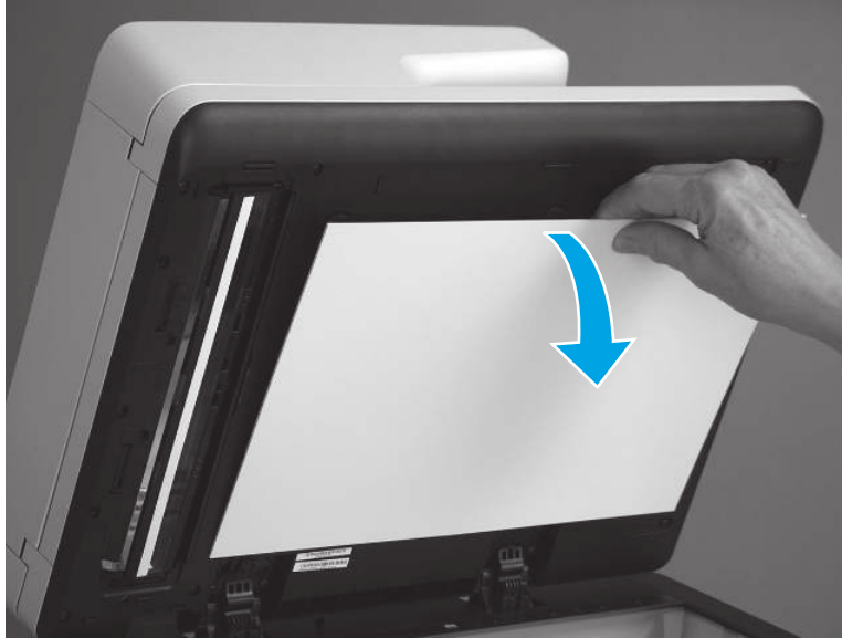
Figure 4-88 Remove the white backing
