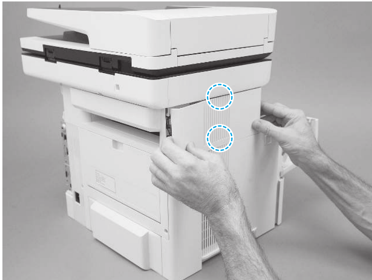
Figure 4-1024 Release two tabs
