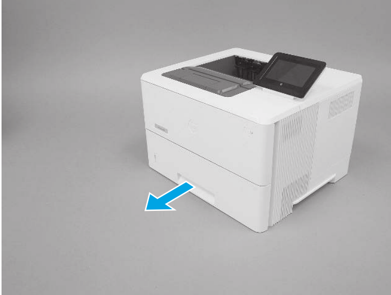
Figure 3-133 Pull the tray out until it stops
