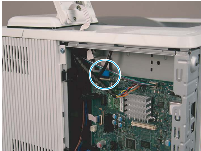
Figure 4-78 Disconnect one FFC (M507/E50145)
