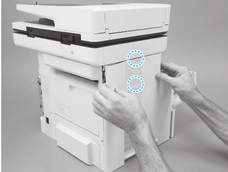
Figure 4-1311 Release two tabs
