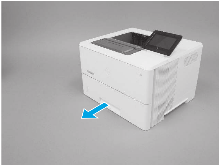
Figure 4-224 Pull the tray out until it stops
