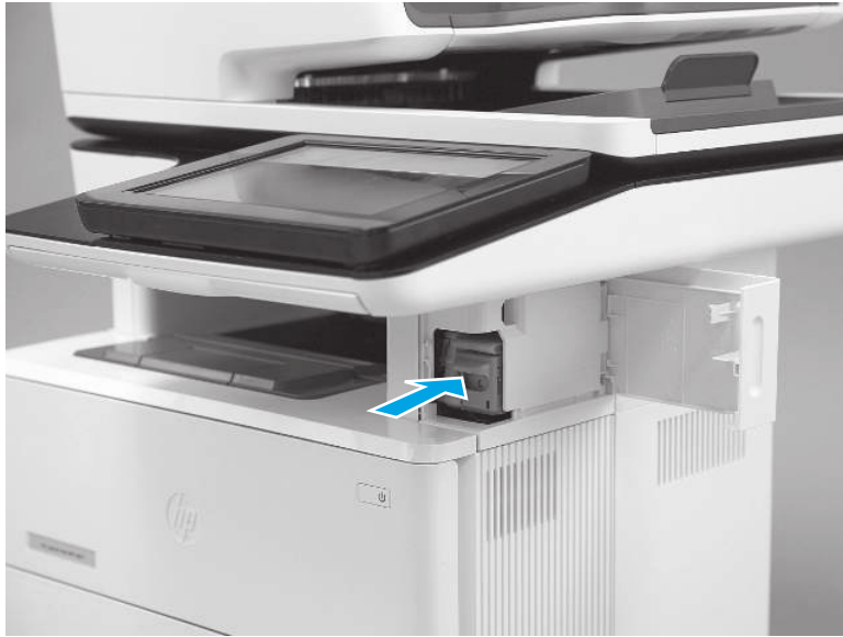
Figure 4-11 Install the staple cartridge
