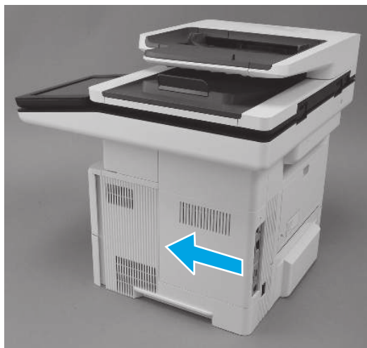
Figure 4-1431 Install the formatter cover (M506/E50045/M507/E50145/M527/E52545/M528/E52645)
