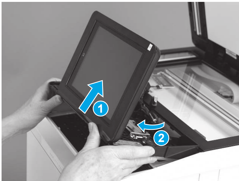
Figure 4-403 Remove the control panel
