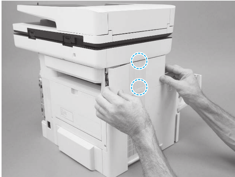
Figure 4-636 Release two tabs
