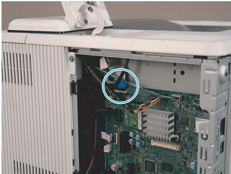
Figure 4-1191 Disconnect one FFC (M507/E50145)
