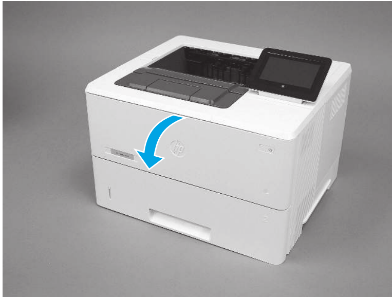
Figure 3-119 Open the toner-cartridge door
