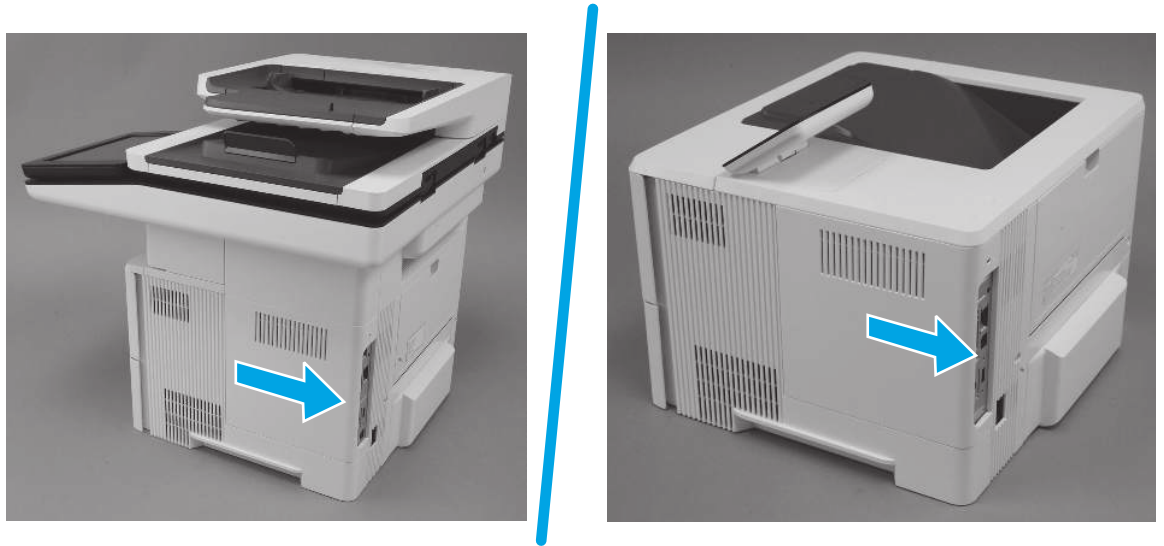
Figure 4-545 Remove the formatter cover (M506/E50045/M507/E50145/M527/E52545/M528/E52645)
