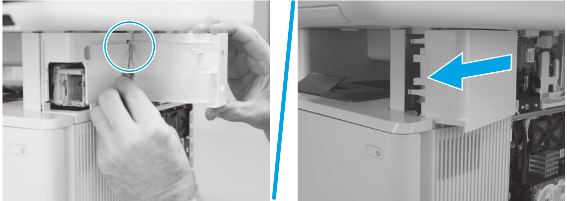
Figure 4-1303 Release the upper hinge or remove the cover
