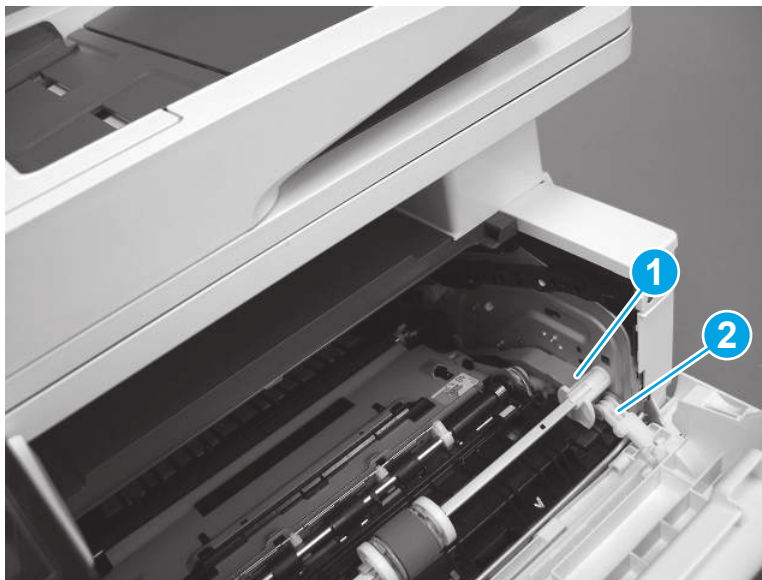
Figure 4-1037 Release the pressure-release link
