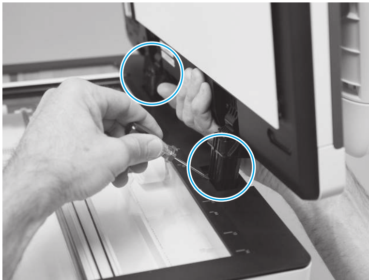
Figure 4-148 Release two tabs
