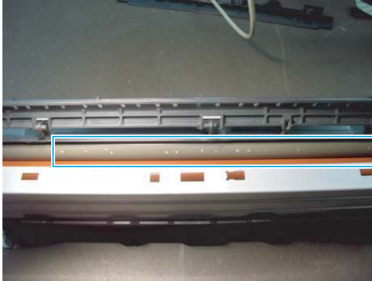
Figure 3-108 Contaminated fuser film
