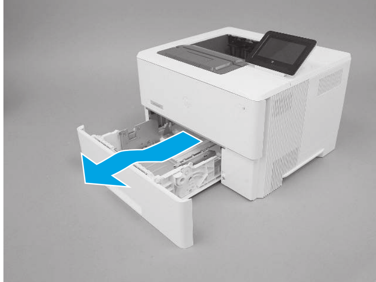
Figure 4-722 Release and remove the tray
