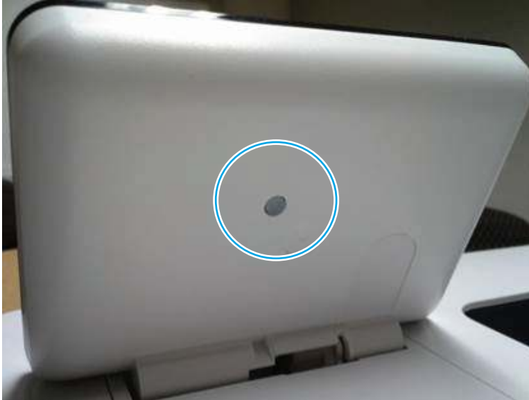
Figure 3-27 Diagnostic-tests access button (M507x and E50145dn)
