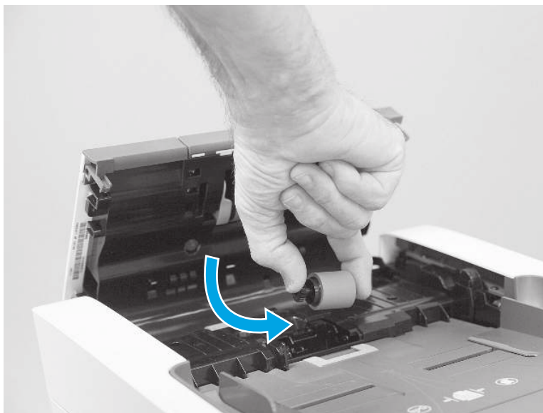
Figure 4-1412 Install the roller assembly
