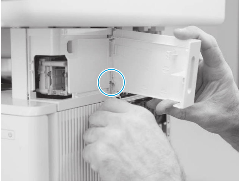
Figure 4-1017 Release the lower hinge
