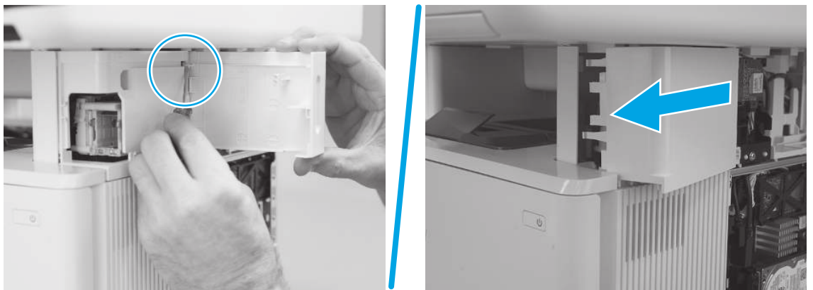
Figure 4-820 Release the upper hinge or remove the cover
