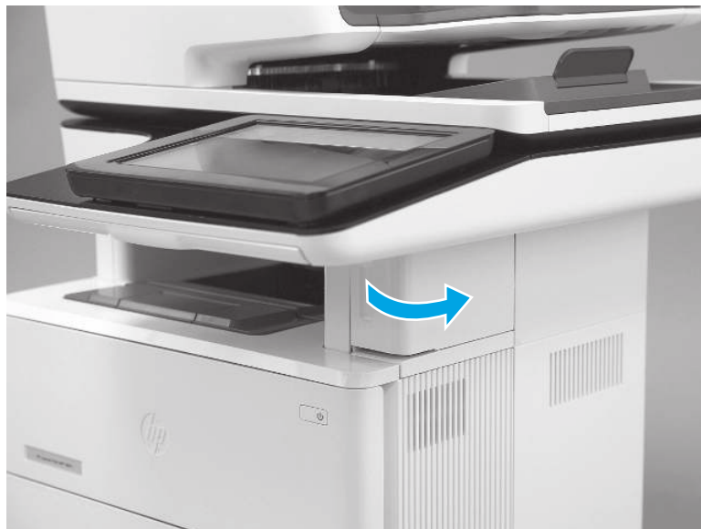
Figure 4-9 Open the stapler door
