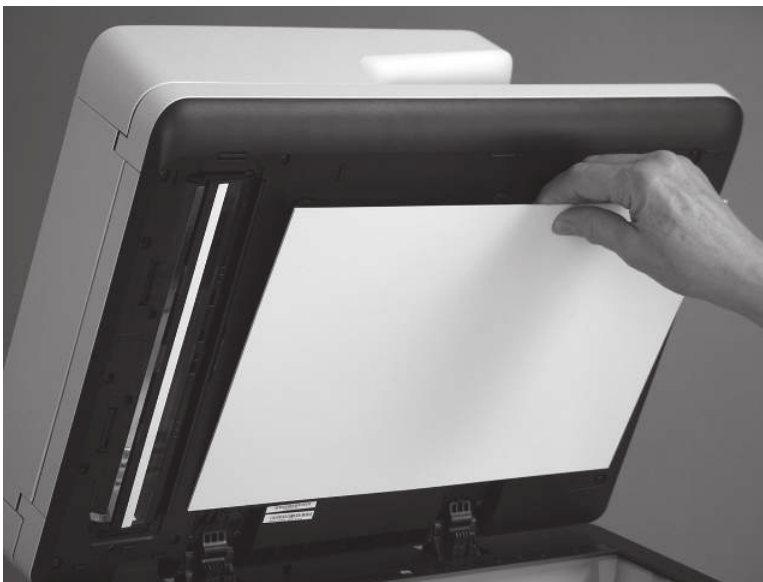
Figure 4-448 Check the white backing
