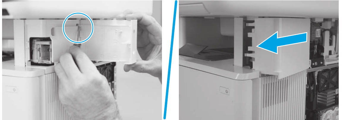
Figure 4-733 Release the upper hinge or remove the cover
