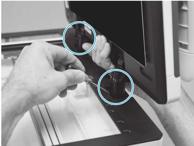
Figure 4-435 Release two tabs
