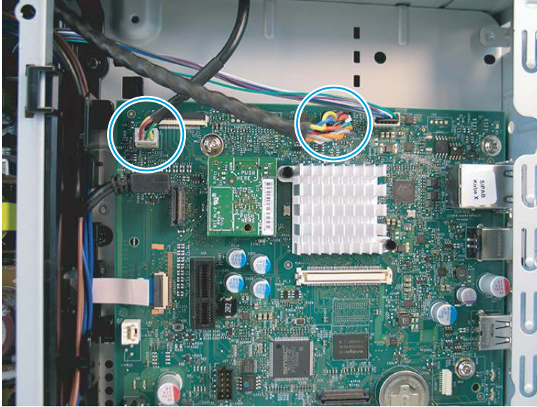
Figure 4-870 Disconnect two connectors
