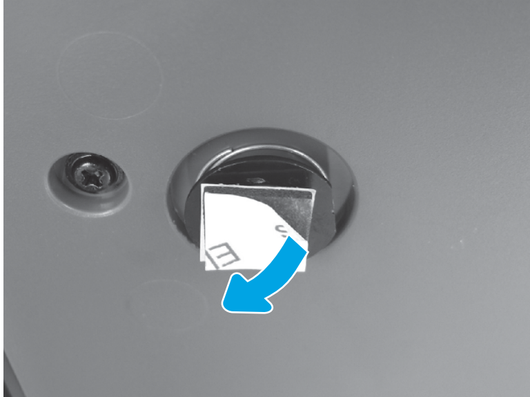
Figure 4-445 White backing adhesive squares
