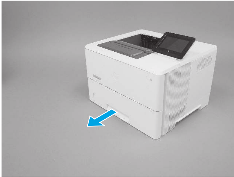
Figure 4-808 Pull the tray out until it stops
