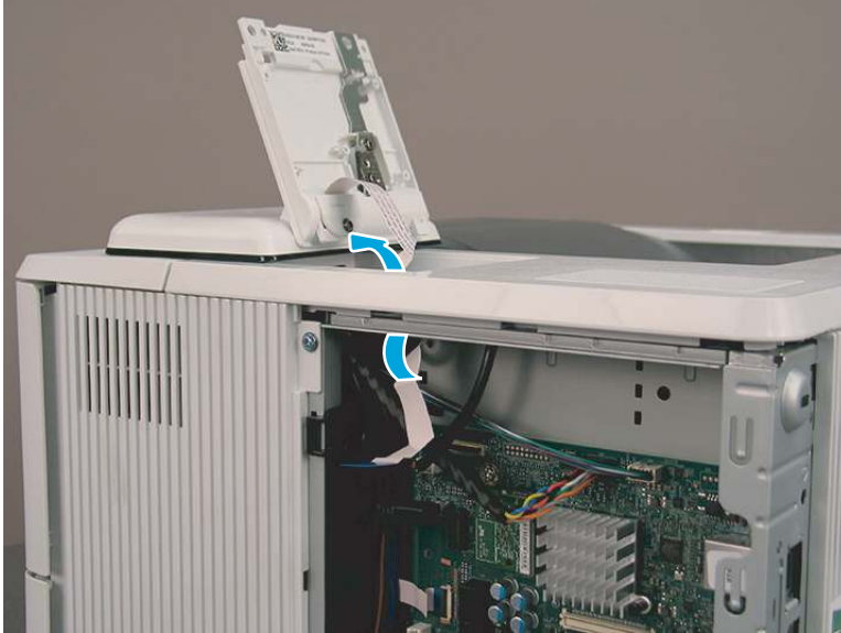
Figure 4-1290 Remove the control panel (M507/E50145)
