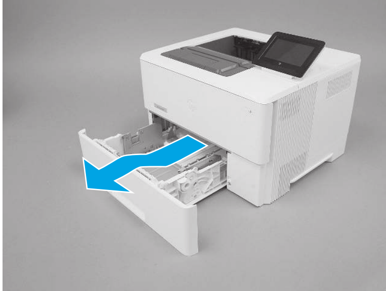
Figure 4-1292 Release and remove the tray
