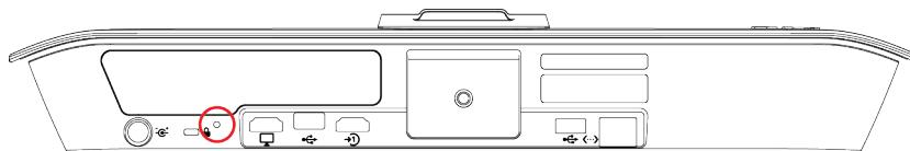
3 While continuing to hold the restore button, reconnect the power supply to turn the system on.
