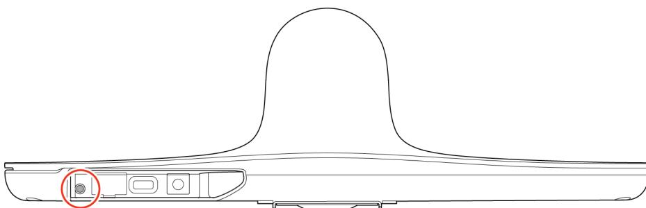
3 While continuing to hold the restore button, reconnect the power supply to turn the system on.
