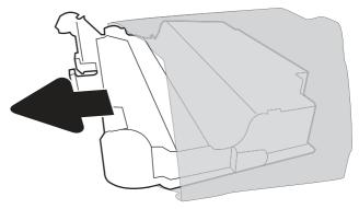
5. Install the new unit into the printer. Make sure the toner-collection unit is firmly in place.
