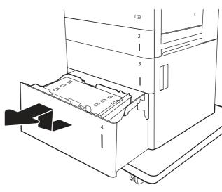
6. If jammed paper is in the feed area, pull it down to remove it. First pull the paper to the left to release it, and then pull it forward to remove it.
