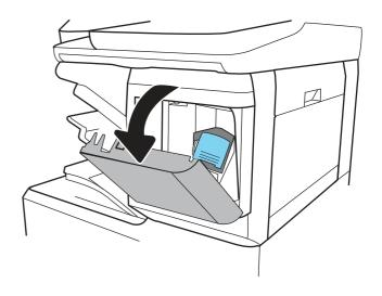
2. Grasp the colored tab on the staple cartridge, and then pull the staple cartridge straight out.
