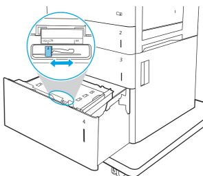
3. Rotate the paper-stop lever to the correct position for the paper being used.
