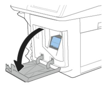
2. Grasp the colored tab on the staple cartridge, and then pull the staple cartridge straight out.
