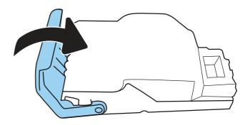
5. Insert the staple cartridge into the stapler and press the colored handle toward the printer until it snaps into place.
