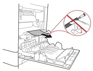
11. If paper is jammed as it enters the output bin, gently pull the paper out to remove it.
