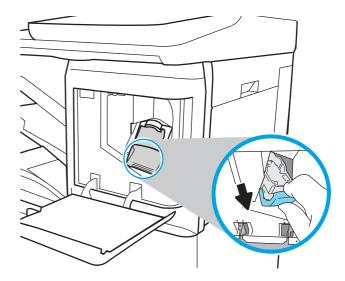
3. Lift up on the small lever at the back of the staple cartridge. Remove the jammed staples.
