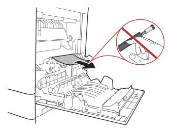
4. If paper is jammed as it enters the output bin, gently pull the paper out to remove it.
