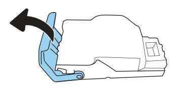
4. Close the lever at the back of the staple cartridge. Be sure that it snaps into place.
