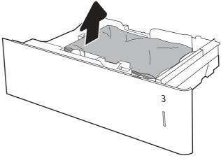
3. Remove any paper from the feed rollers inside the printer. First pull the paper to the left to release it, and then pull it forward to remove it.
