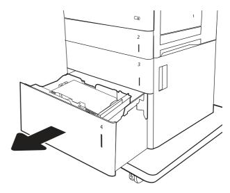
2. Remove any jammed or damaged sheets of paper. Verify that the tray is not overfilled and that the paper guides are adjusted correctly.
