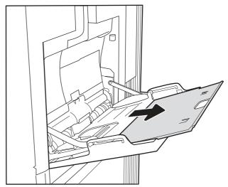
Use the blue adjustment latch to spread the paper guides to the correct size, and then load paper in the tray. For information about how to orient the paper, see Table 2-1 <u>Tray 1 paper orientation on</u> page 21
