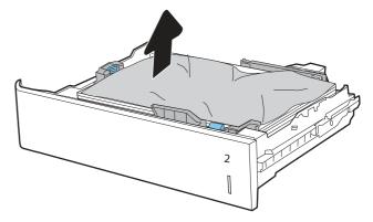
3. Gently remove any paper from the feed rollers inside the printer. First pull the paper to the left to release it, and then pull it forward to remove it.
