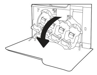
2. Grasp the handle of the used toner cartridge and pull out to remove it.
