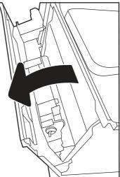
3. Grasp the top of the toner-collection unit and remove it from the printer.
