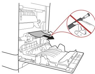
8. If paper is jammed as it enters the output bin, gently pull the paper out to remove it.
