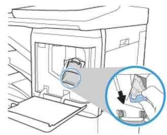
3. Remove the staple cartridge from the sled and replace it with the new staple cartridge.
