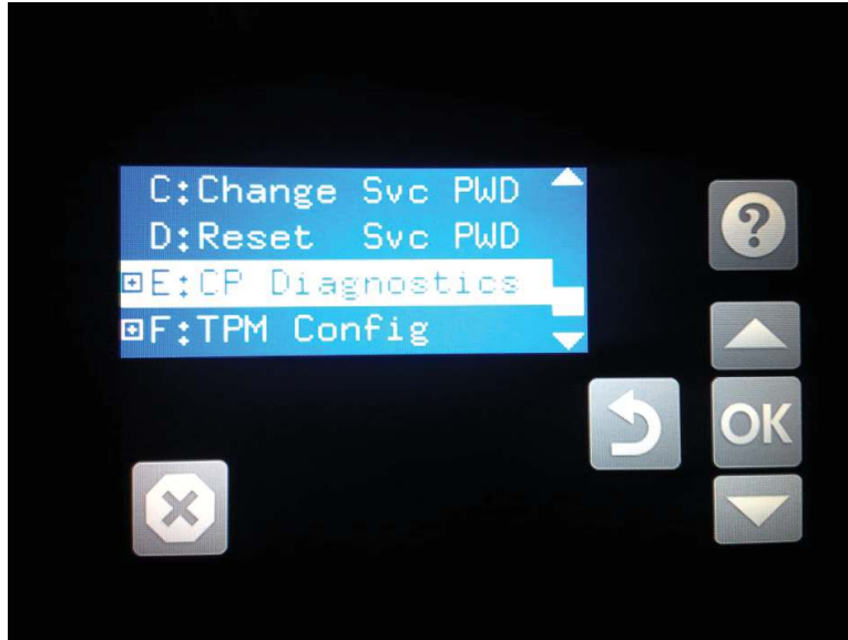
Figure 3-34 Access the diagnostics menu
