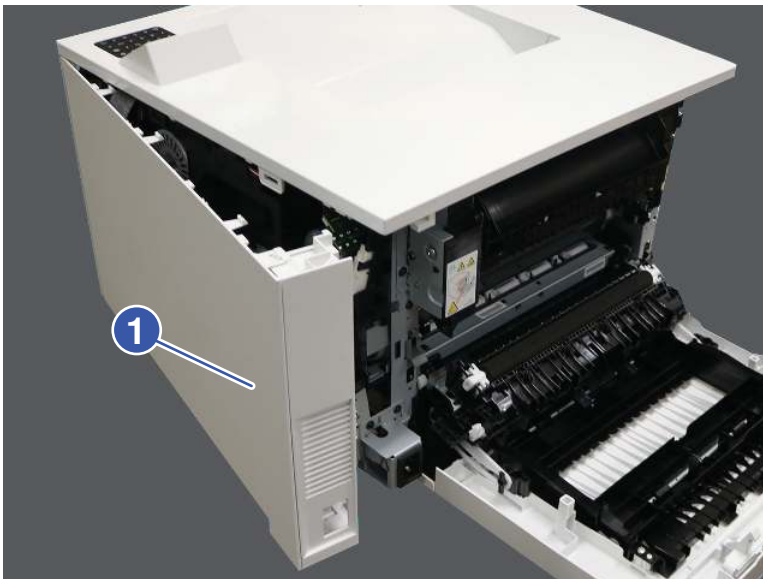
Figure 4-262 Remove the cover
