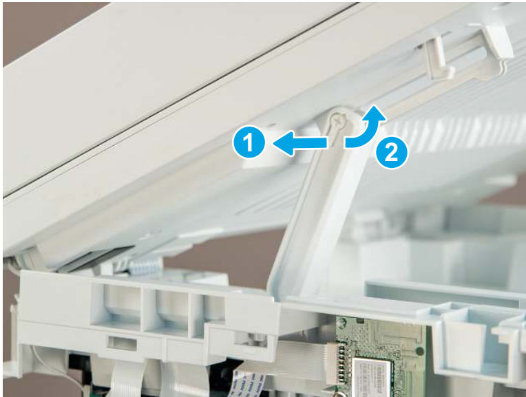
Figure 4-24 Release the slider pin
