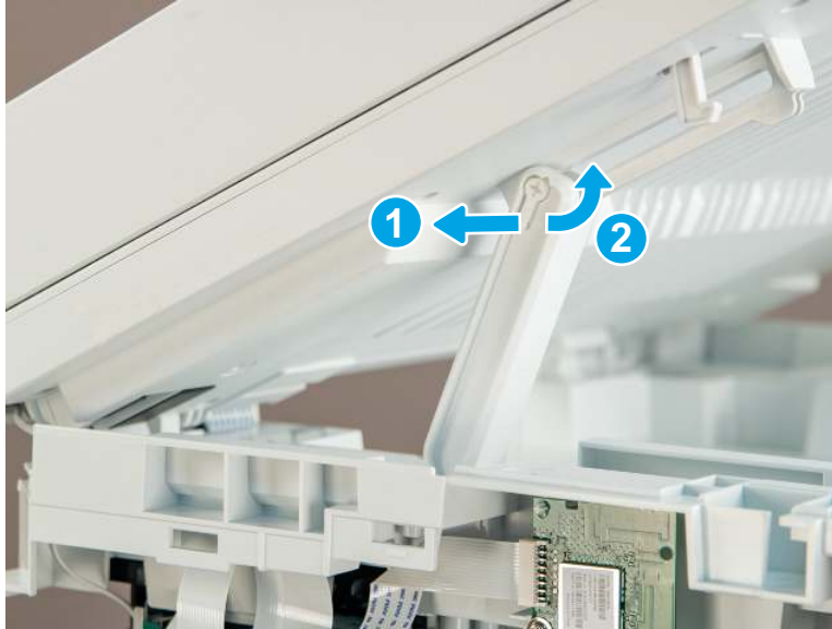
Figure 4-111 Remove the slider pin
