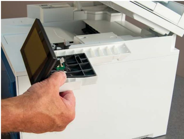
Figure 4-39 Remove control panel and mount base
