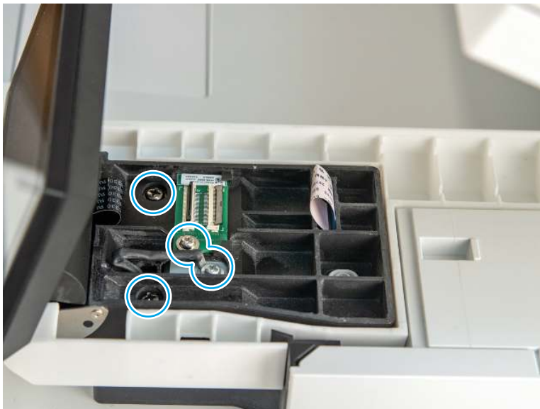
Figure 4-37 Remove four screws
