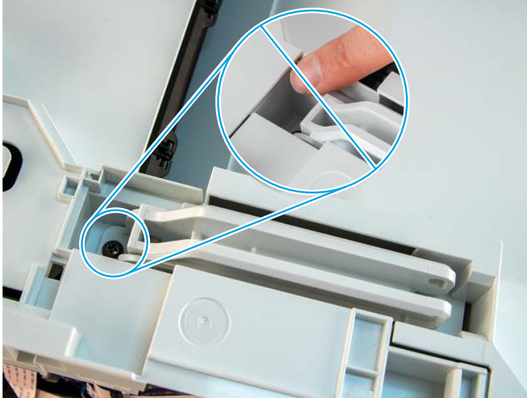
Figure 4-719 Remove one screw
