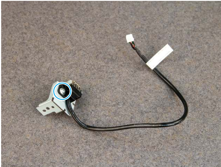
Figure 4-193 Separate the assembly from the bracket
