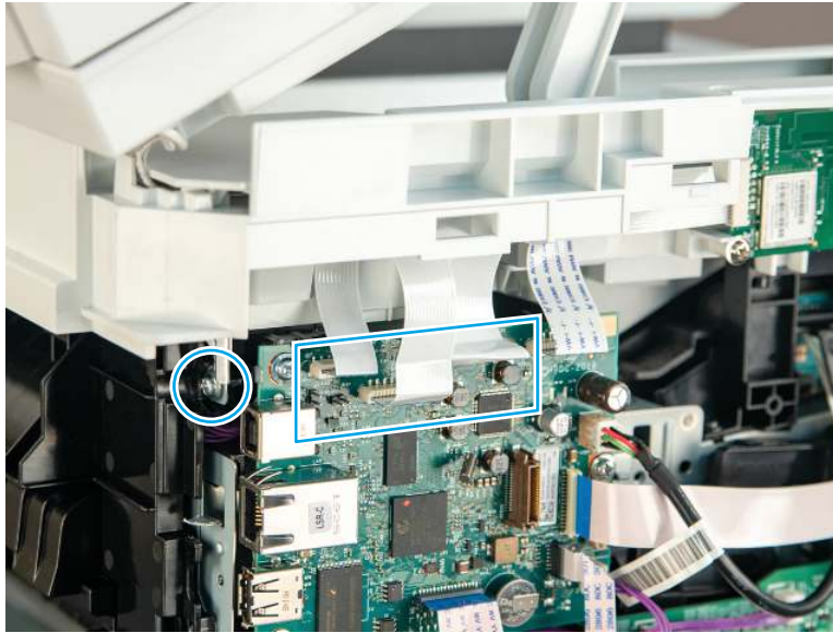
Figure 4-691 Disconnect FFCs and remove screw
