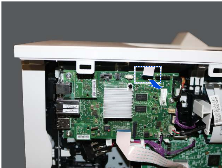
Figure 4-502 Disconnect one flat-flexible cable
