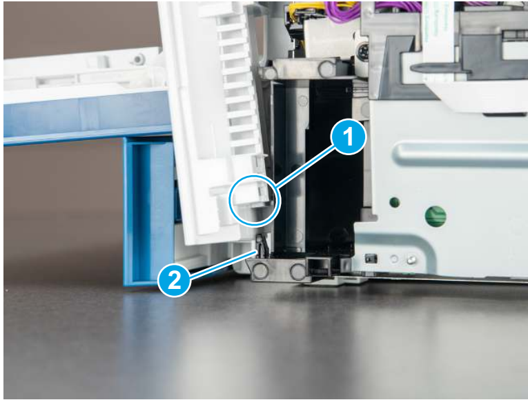
Figure 4-448 Cover alignment pins
