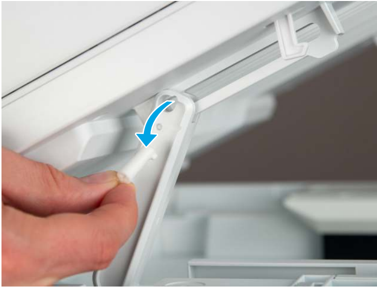
Figure 4-25 Remove the slider pin
