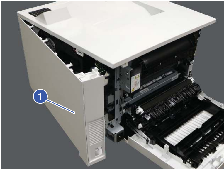
Figure 4-302 Remove the cover
