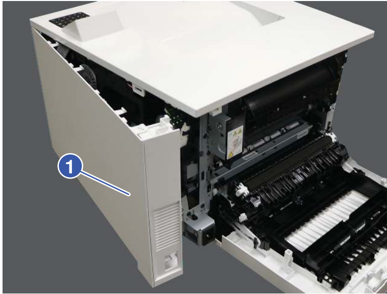
Figure 4-55 Remove the cover
