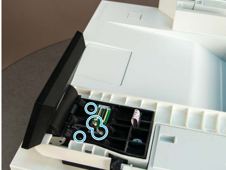
Figure 4-187 Remove four screws
