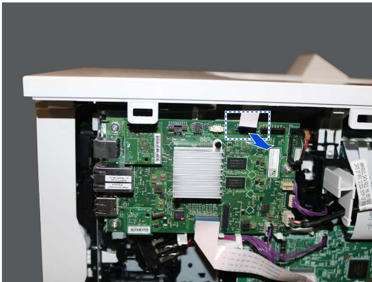
Figure 4-643 Disconnect one flat-flexible cable
