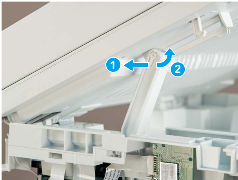
Figure 4-692 Remove the slider pin
