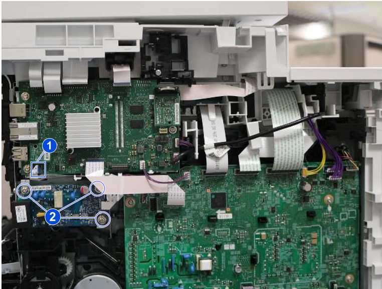
Figure 4-661 Remove the fax PCB
