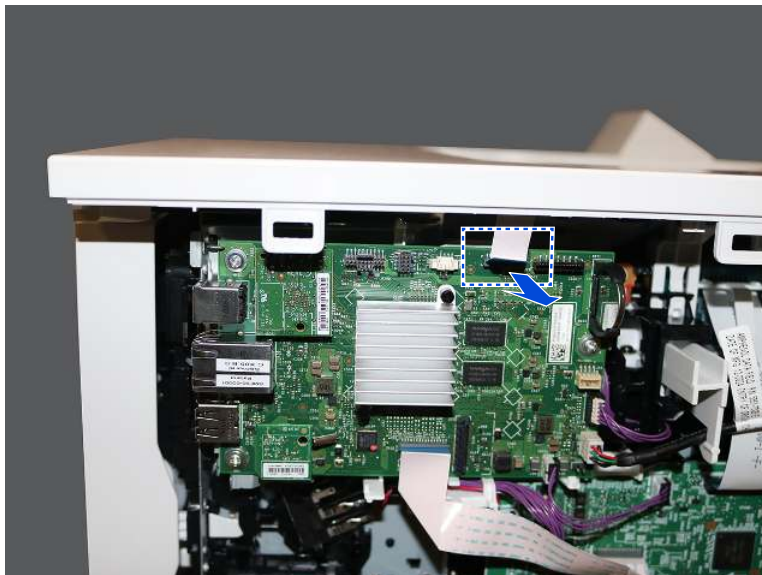
Figure 4-96 Disconnect one flat-flexible cable
