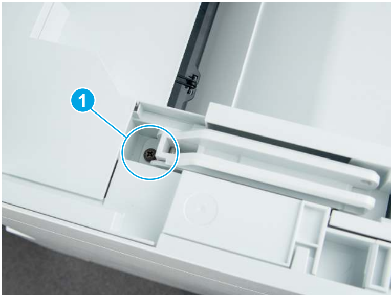
Figure 4-28 Remove one screw
