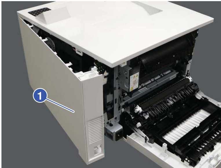
Figure 4-702 Remove the cover
