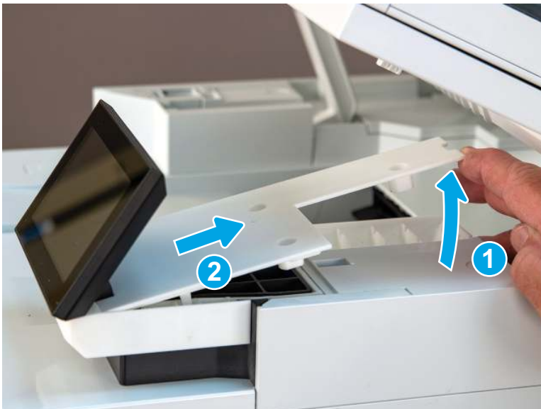
Figure 4-35 Remove the cover
