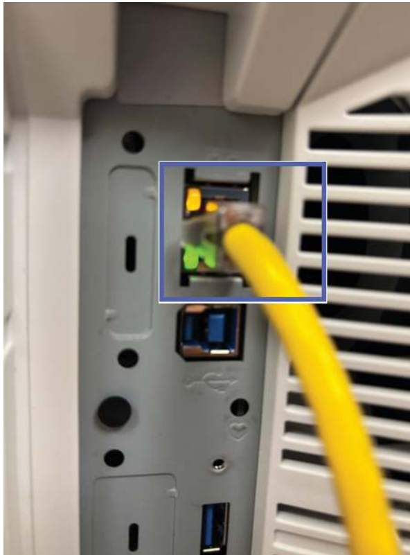
Figure 3-52 Yellow and green LEDs on the network port
