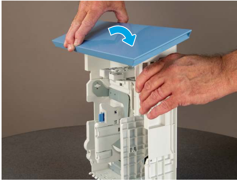
Figure 4-1061 Install the cover
