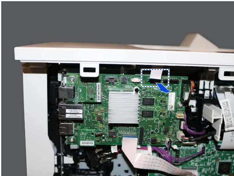
Figure 4-714 Disconnect one flat-flexible cable
