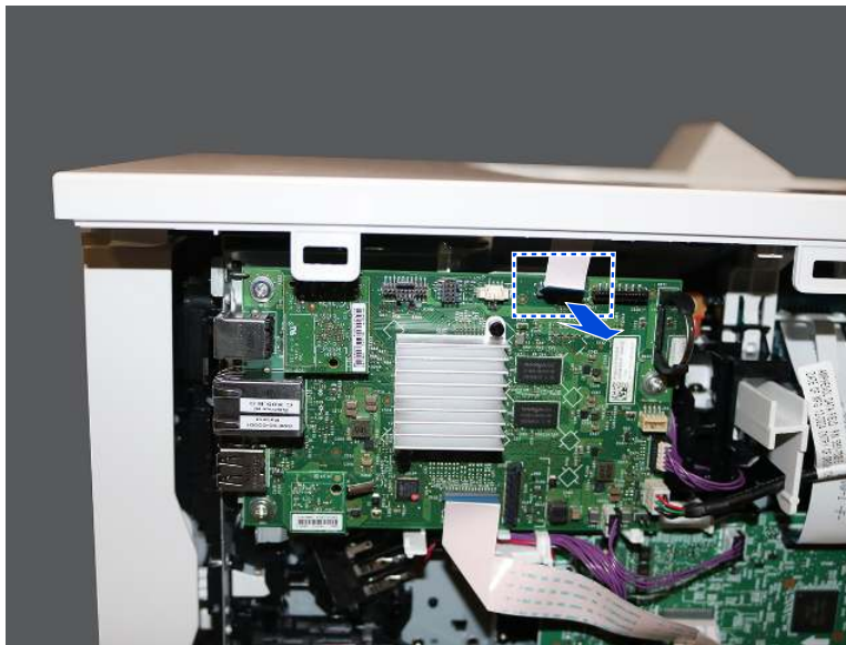
Figure 4-309 Disconnect one flat-flexible cable
