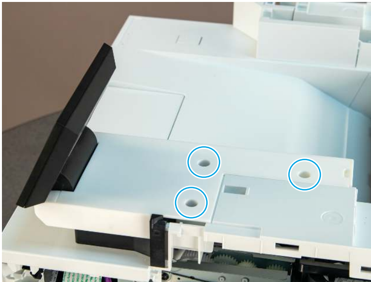
Figure 4-594 Remove three screws
