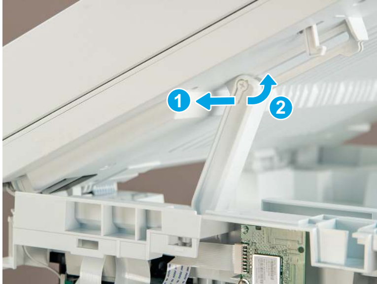
Figure 4-626 Remove the slider pin
