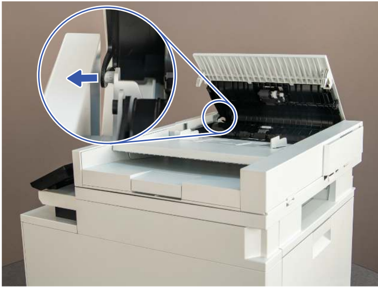
Figure 4-2 Release the clip
