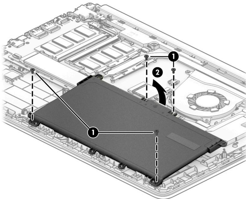
To insert the battery, reverse the removal procedures.
