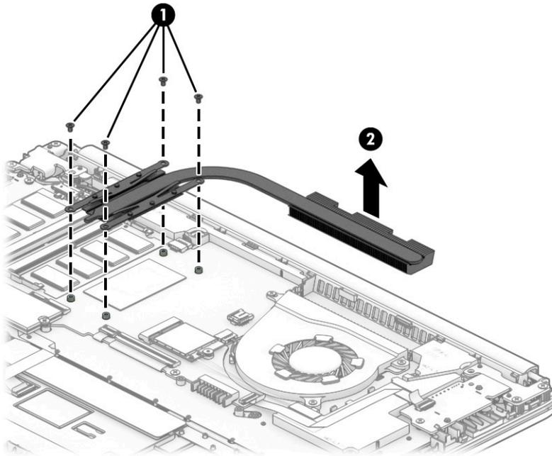
3. Apply thermal grease to the integrated processor on the system board **(1)** and associated location on the heat sink **(2)**.
