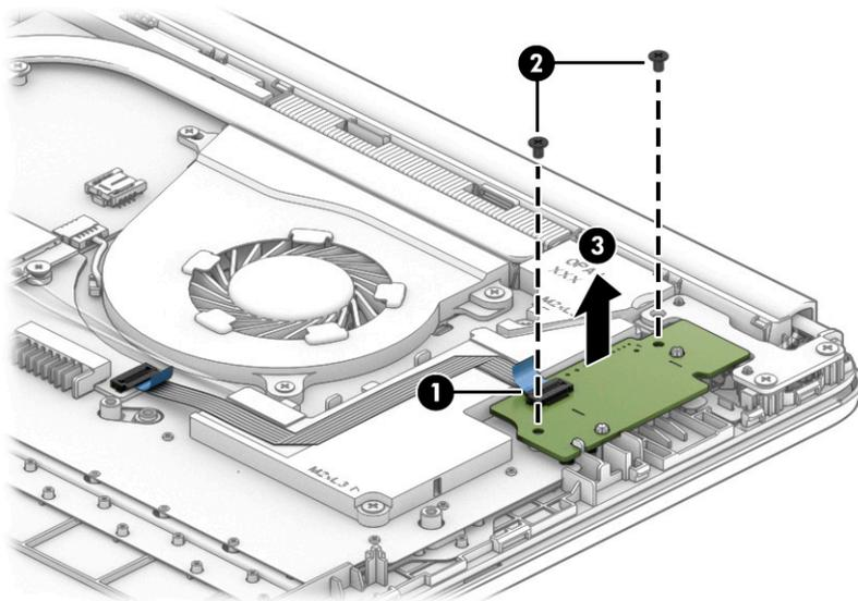
Reverse this procedure to install the power button/card reader board.
