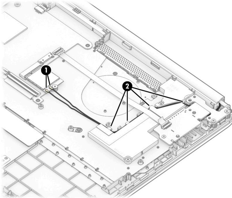
2. Disconnect the speaker cable from the system board **(1)**.
