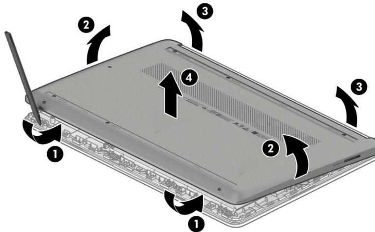
To replace the bottom cover, reverse the removal procedures.
