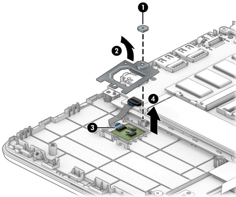
Reverse this procedure to install the fingerprint reader board.
