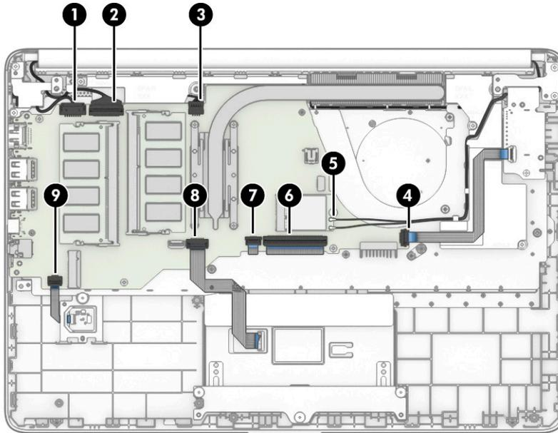
2. Remove the four Phillips M2.0 × 2.0 screws **(1)** that secure the system board to the computer.
