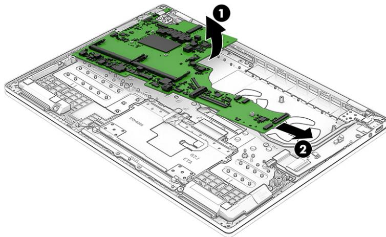
6. If you are replacing the system board, remove the USB bracket from the old system board and install it on the new system board.
