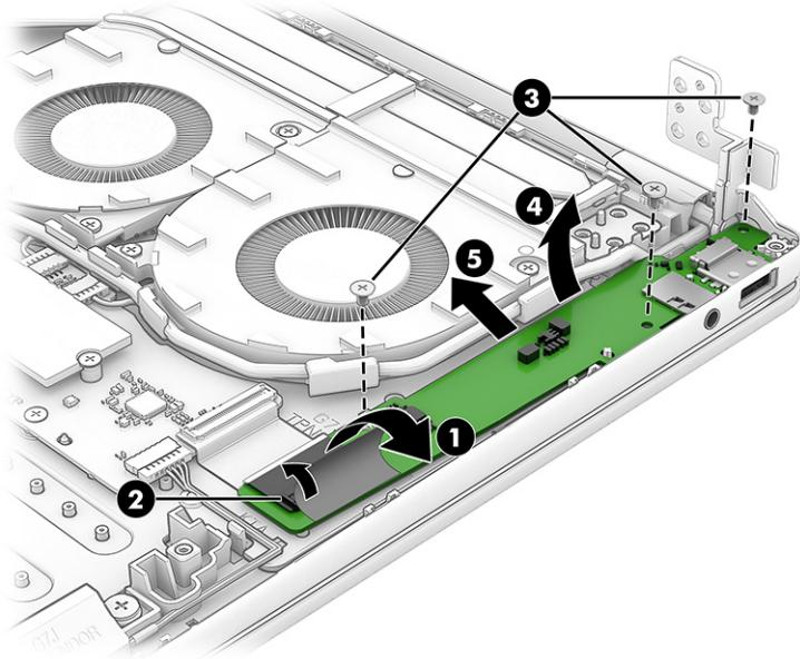
To install the I/O board, reverse this procedure.
