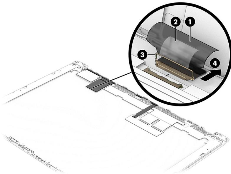
**13.** To remove the display power board and cable:
