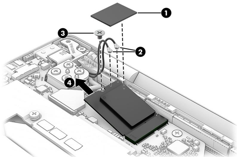
5. If the WLAN antenna is not connected to the terminal on the WLAN module, install a protective sleeve on the antenna connector, as shown in the following illustration.
