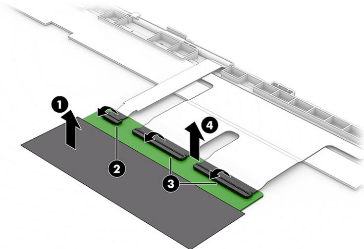
**16.** To remove the camera module:
