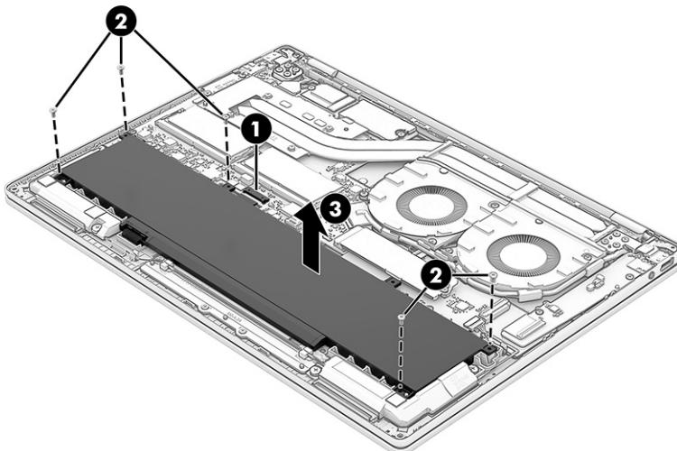
To reinstall the battery, reverse the removal procedures.
