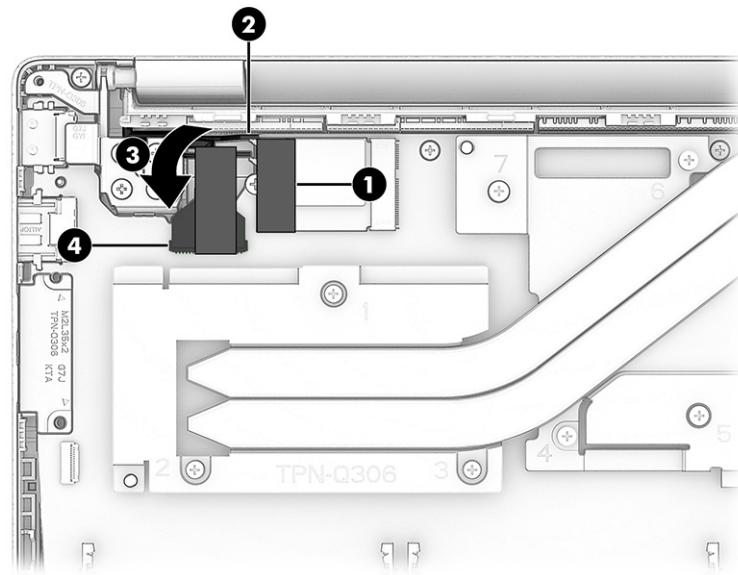
5. Lift the tape (1) off the display connector.
