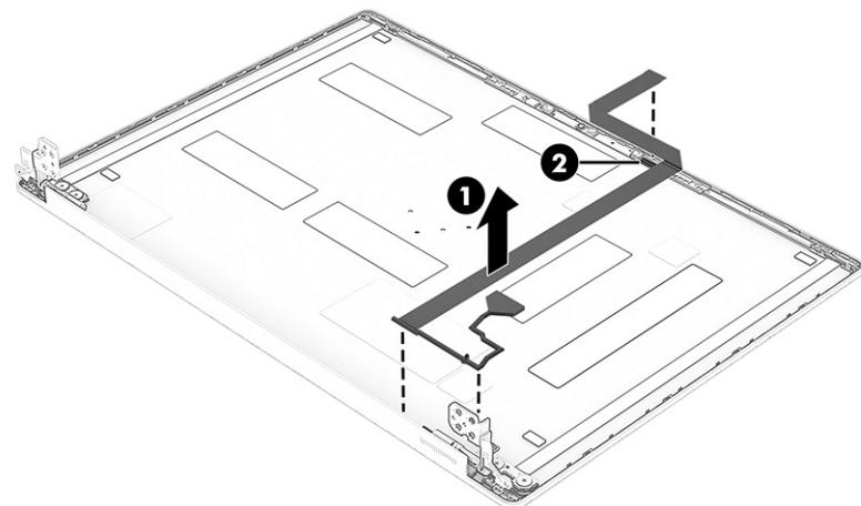
c. Note the alignment marks when installing a camera cable.
