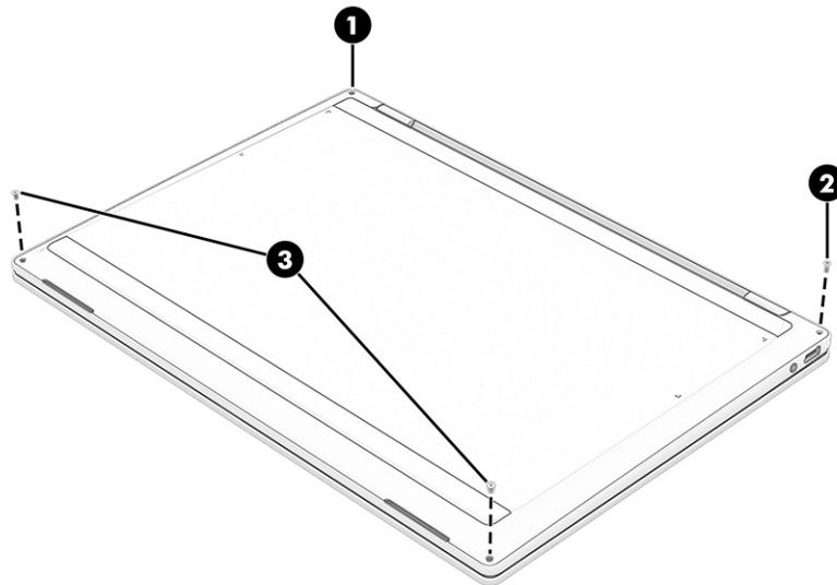
5. Insert a tool **(1)** near the captive screw to release the cover.
