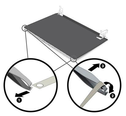
e. Release the left and right sides (1) of the panel, and then pull the panel (2) up and away from the rear cover.
