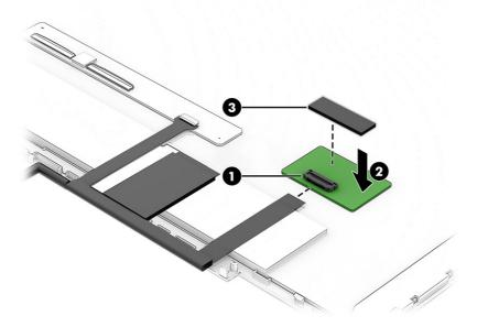
q. Install foil onto the display panel. Be sure the apply the foil smoothly, as it cannot be tilted or wrinkled. Align the right side of the foil with the seam on the bezel.
