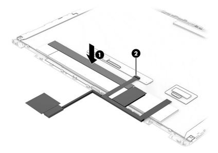
m. Install stretchable tape onto the bottom of the OLED board up against but not covering the bare copper area behind the OLED board.
