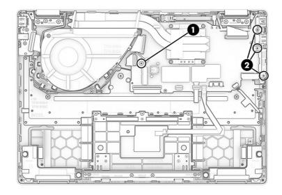
4. Lift the left side of the system board (1) up, and then pull the board (2) to the left to remove it from the computer.
