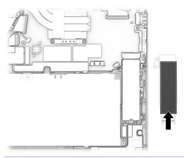
NOTE: SSDs are designed with a notch to prevent incorrect insertion.
