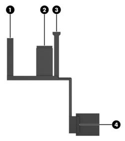
b. To install the touch control board, install stretchable tape (1) onto the back of the board while aligning the holes (2) in the tape with the holes on both sides of the board.
