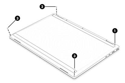
5. Insert a tool (1) into the seam near the top left hinge computer and release the cover.
