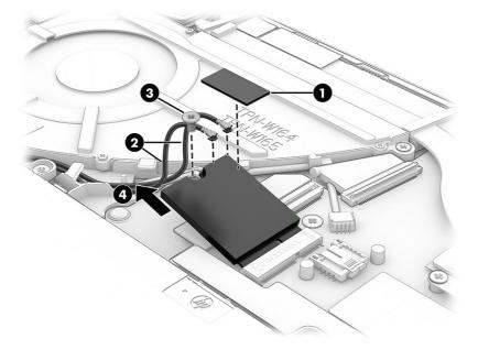
5. If the WLAN antenna is not connected to the terminal on the WLAN module, install a protective sleeve on the antenna connector, as shown in the following illustration.
