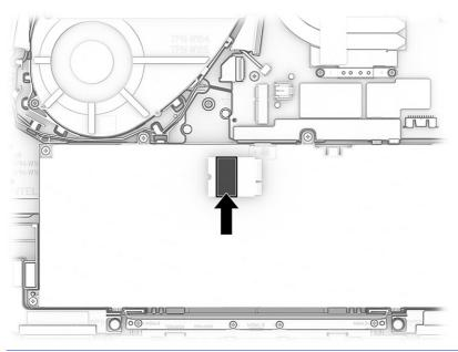
NOTE: WLAN modules are notched to prevent incorrect installation.
