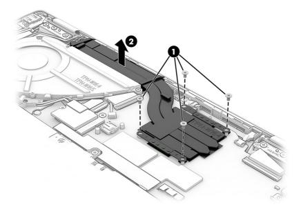
3. Thoroughly clean the thermal paste from the surfaces of the heat sink and the system board components each time the heat sink is removed.
