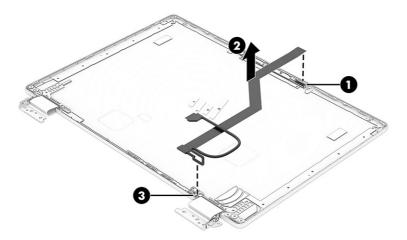
18. To remove the hinges and hinge covers from the display rear cover:
