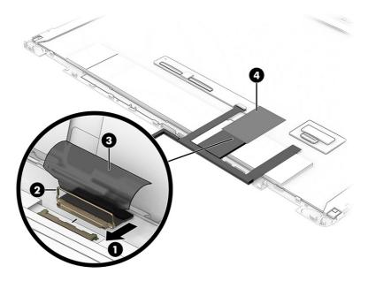
I. Align the long thermal pad with the edge of the OLED cable, and then install the pad (1) from right to left onto the bottom of the display panel. Connect the OLED cable (2) to the touch board.
