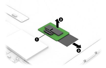
d. When installing an OLED board, be sure that a thermal pad is installed on the board.
