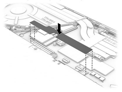
Reinstall the system board cover by positioning the left and bottom sides of the cover up against the right side of the camera connector (1) and the bottom of the WLAN connector (2).
