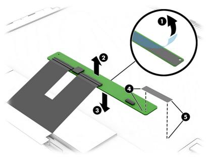
Use the following illustration to determine proper installation. Be sure that:
