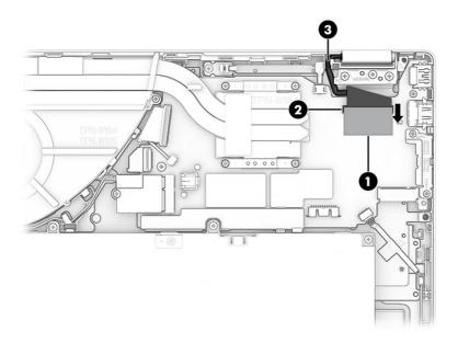
9. Remove the six Phillips M2.5  $\times$  5.0 screws that secure the display assembly to the computer.
